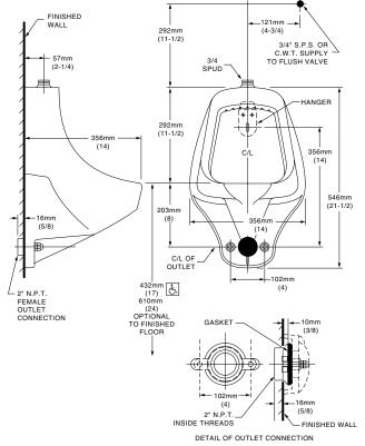
FLUSH VALVE NOT INCLUDED WITH FIXTURE AND MUST BE ORDERED SEPARATELY. PROVIDE SUITABLE REINFORCEMENT FOR ALL WALL SUPPORTS.
